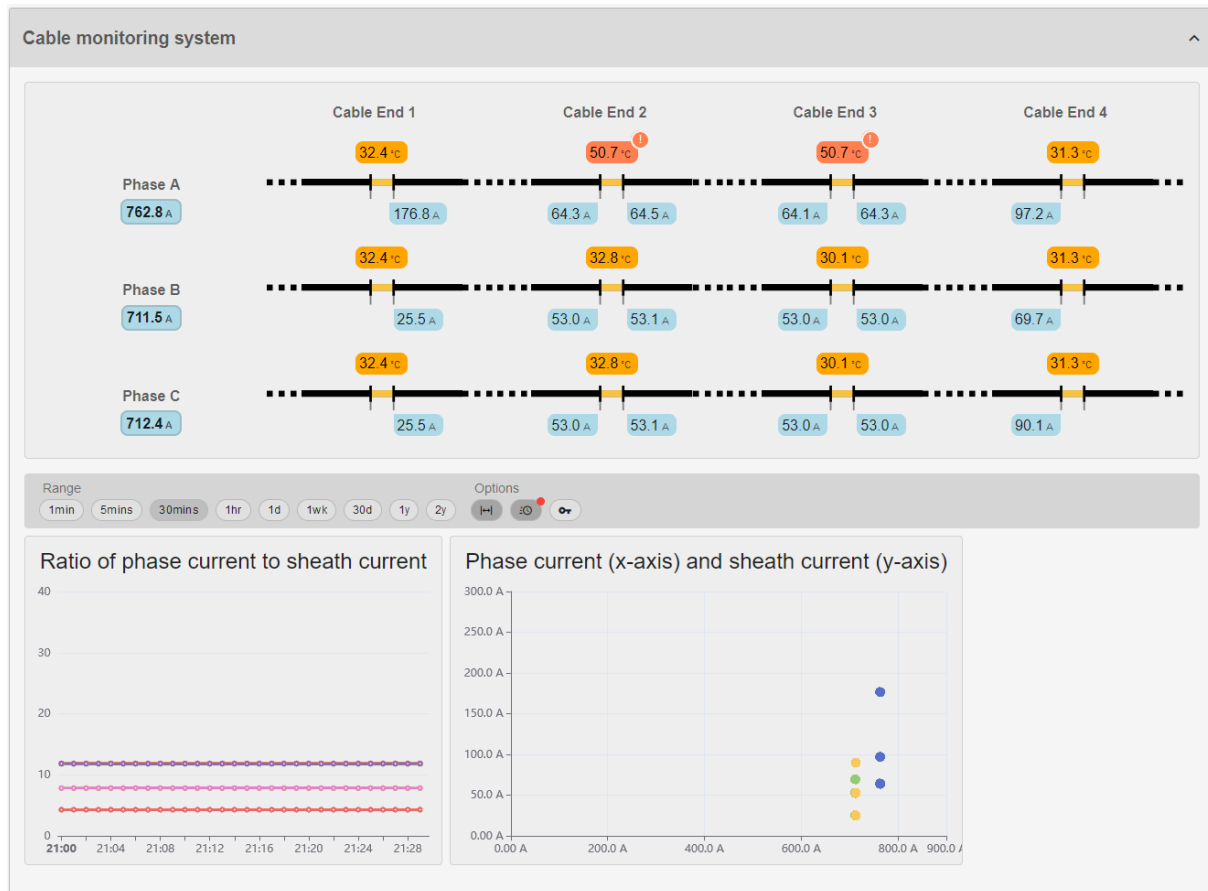
Figure 10: Cable asset monitoring view (using simulated data)
