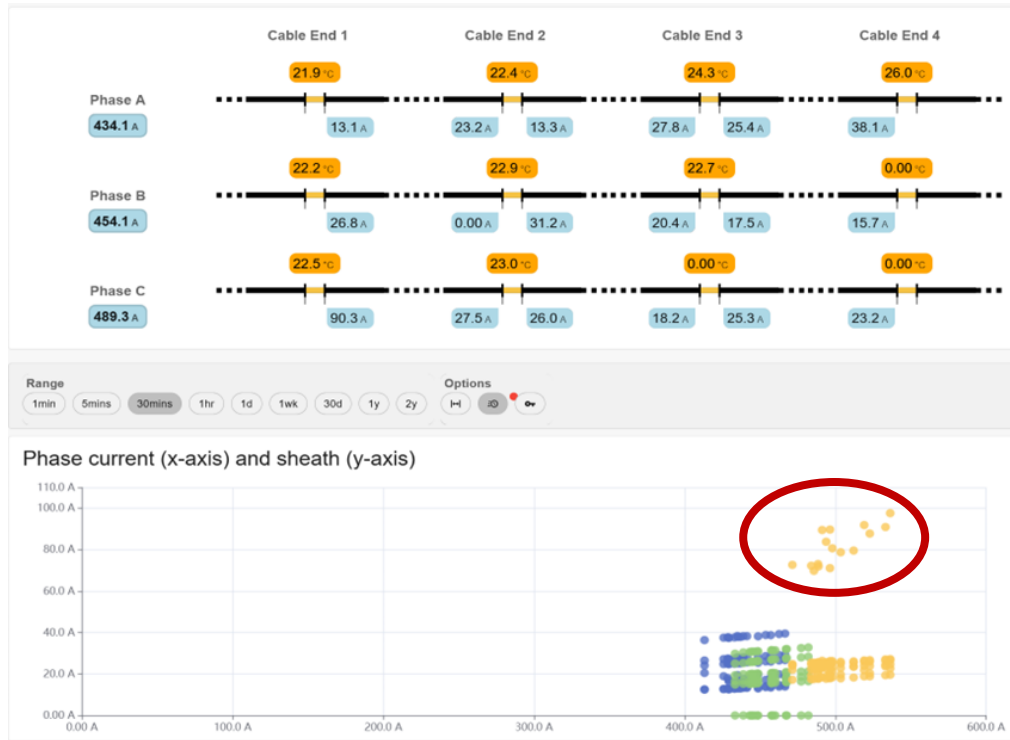
Figure 8 – Outliers detected in ratio of phase to sheath current
