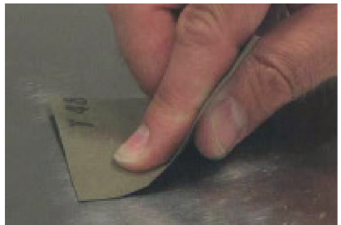
Figure 2.3: Roughening the surface of the measuring object
