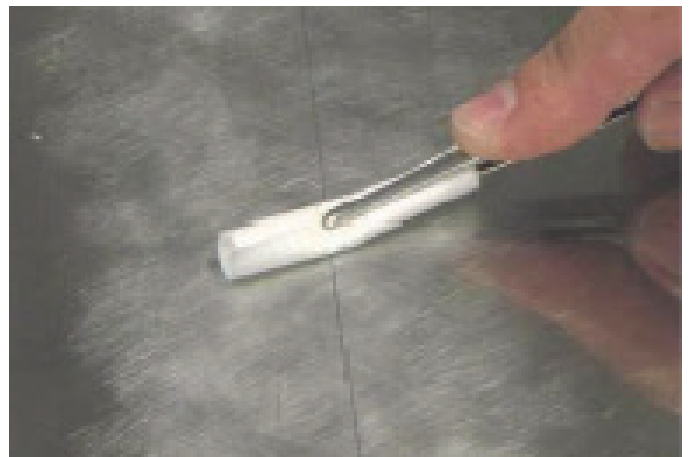
Figure 2.8: Final cleaning of the installation point
