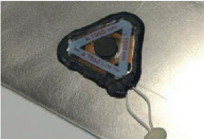
Figure 2.21: Covering the sensors edges with AK22
