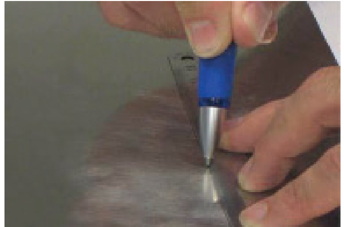
Figure 2.7: Marking the marking lines
