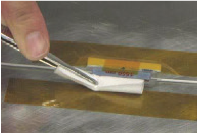
Figure 2.13: Removing the excess adhesive
