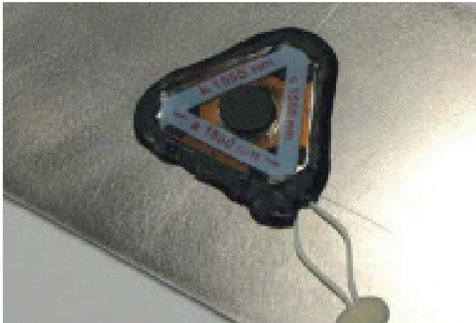
Figure 2.21: Covering the sensors edges with AK22
